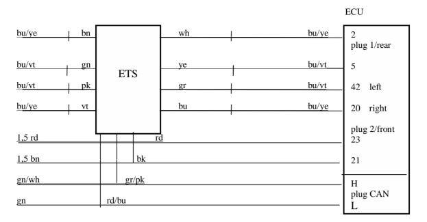
The CAN-plug is a 2-pole plug and sits between plug 1 and plug 2.
